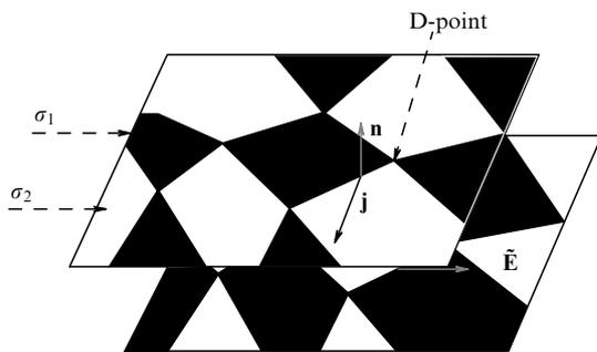
**Figure 1.** Two-phase dual medium. At the top is the ‘parent’ medium, and at the bottom is the dual medium, with  $\mathbf{n}$  being a unit vector normal to the plane of the medium. The dashed arrow points to one of the D-points. The area with conductivity  $\sigma_1$  ( $\sigma_2$ ) in the ‘parent’ medium corresponds to the area with  $\sigma_2$  ( $\sigma_1$ ) in the dual medium.
