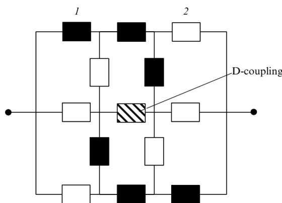
**Figure 6.** One possible implementation of a finite-size D-network [15]. Black rectangles stand for resistors  $z_1$ , and white rectangles stand for resistors  $z_2$ . At the center of the network there is a D-coupling, which in order to meet the network variant of the transformations (2) and (3) and the condition  $\tilde{\sigma}_e = \sigma_e$  must have a resistance equal to  $\sqrt{z_1 z_2}$ . The D-coupling (resistor) is a network analog of D-points in the continuous case (see Fig. 1).
