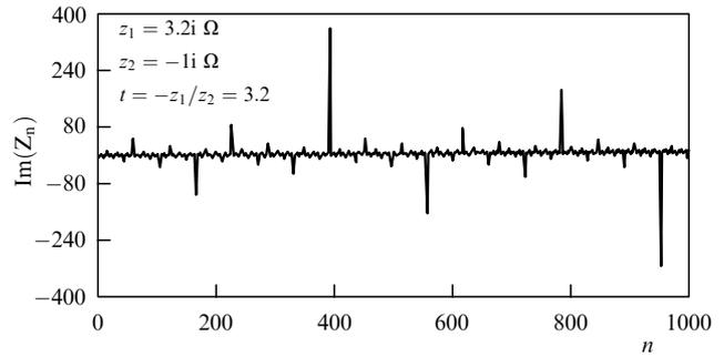
Figure 9. Chaotic dependence of the impedance of a ladder-type circuit on the number  $n$  of elements. The parameter  $t$  is selected equal to  $-z_2/z_2 = 3.2$  and, according to the criterion (28), is within the instability range.
